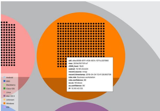
Figure 3. The same network as shown in Figure 2, but zoomed into a specific inner circle and hovered over a specific device to view additional metadata that Poseidon learned about it.
